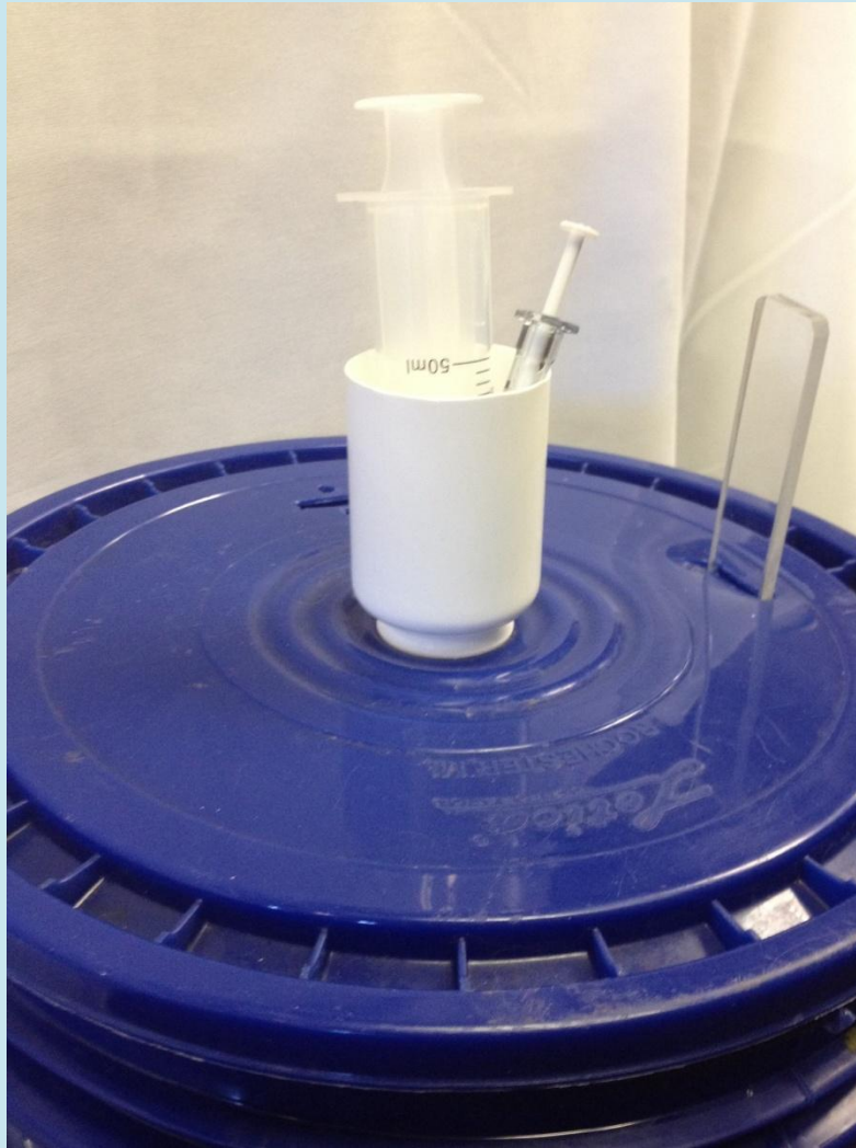
“Agitator”, Sawyer filter plunger, and chlorine syringe resting positions when bucket not in use.
